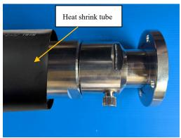
**Step 12:** Slide heat shrink over connector as shown. Using mapp gas or heat generator, apply heat to heat shrink. When heat shrink is installed correctly, adhesive will be visible on each end to the heat shrink. This will ensure proper weather proofing.
