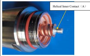
Step 6: Install helical inner contact (A) using a large flat head
