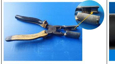
It is recommended to use special plier in **Step 11** to protect plating of connector basket during installation.
