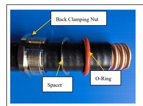
**Step 2:** Install Back Clamping Nut, Spacer and O-Ring onto coax as shown in photo. (Grease O-Ring prior to install).
